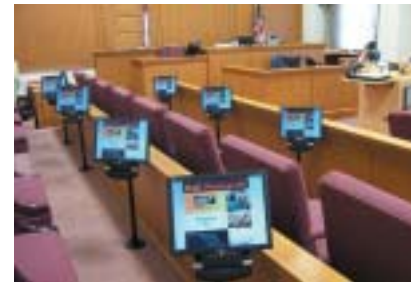
▲ Building on its courtroom evidence presentation offerings, Hall Research initially began to develop its AV over Category 5 technology for a county court in New York. Starting with a Cat-5 matrix switch for that application, eventually customers sought a simple VGA signal out, and the Mini-CAT was born.
